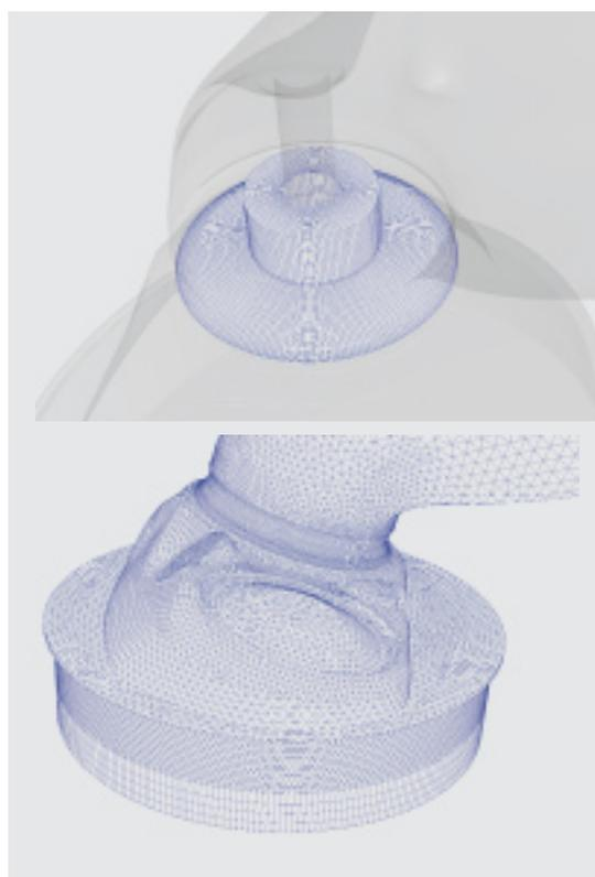
Meshed areas for the valve (top) and combustion chamber (bottom)
