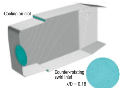
Geometry and mesh for a lean premixed natural gas power turbine CFD case, based on the General Electric Aircraft Engines LM6000 engine
