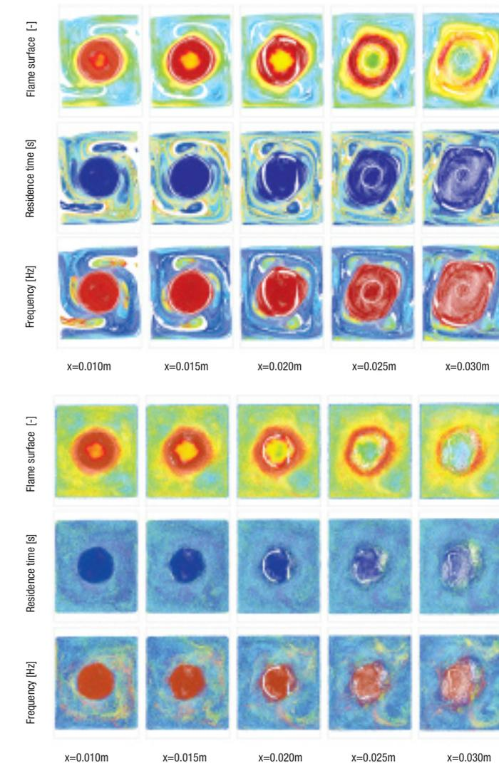
A series of Poincaré planes used in the analysis of a gas turbine case (specifically the GEAE LM6000) modeled using FLUENT software: (top) RANS turbulence model and (bottom) LES turbulence model
