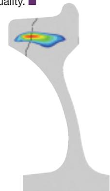
Vertical split rim and contours showing the residual tensile stress
