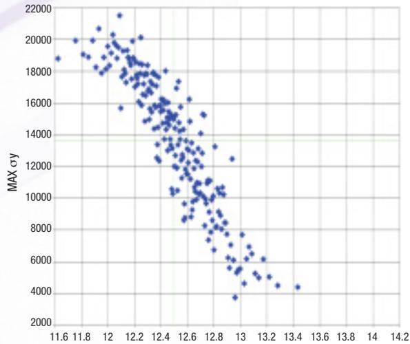
The scatter plot compares maximum axial stress to the stress exponent. Correlation coefficients show strong sensitivity of the stresses to creep.
