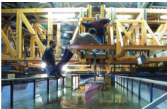
Experimental testing area used to study water flow and wave formation around a boat as well as total drag
