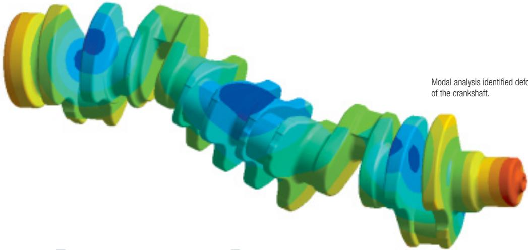
Modal analysis identified deformation of the crankshaft.
