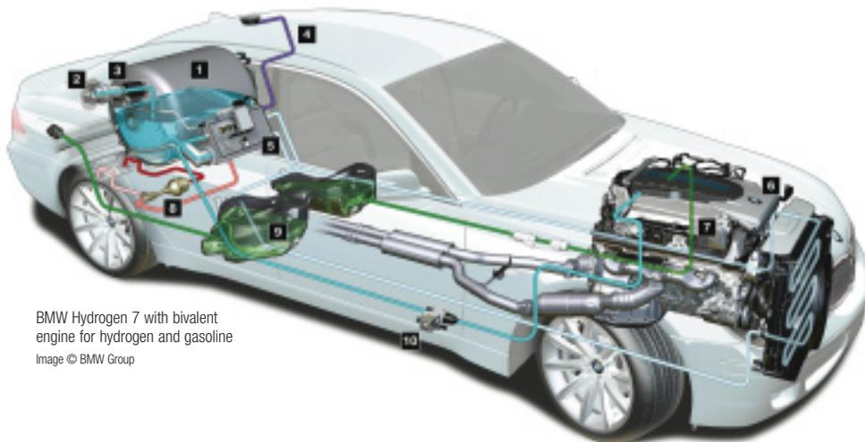
BMW Hydrogen 7 with bivalent engine for hydrogen and gasoline
