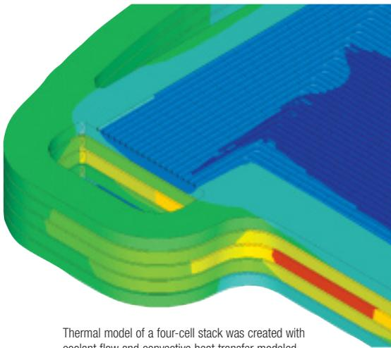
Thermal model of a four-cell stack was created with coolant flow and convective heat transfer modeled with pipe elements. Pipes also were used to model thermal contribution of air and hydrogen flow.
