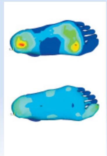
Von Mises stress distributions on the plantar surface of the foot using the flat (top) and total contact insoles (bottom)
