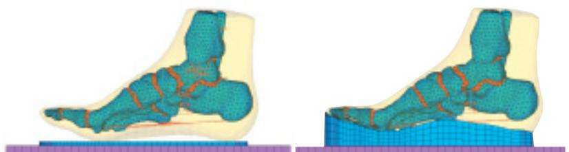
Two insoles, one flat (left) and one shaped to contact the entire sole of the foot (right), were compared in this analysis to understand the impact of the geometry on foot pain.
