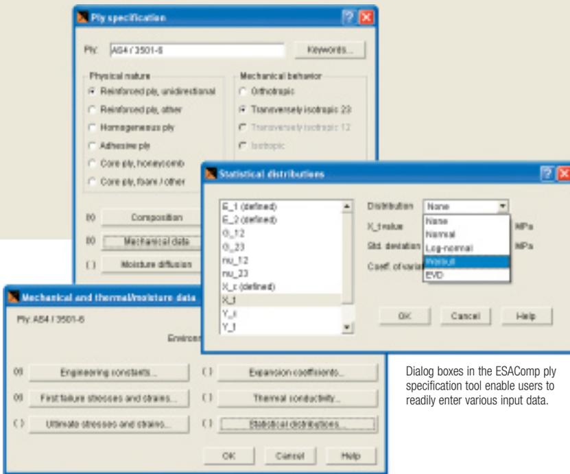
Dialog boxes in the ESAComp ply specification tool enable users to readily enter various input data.
