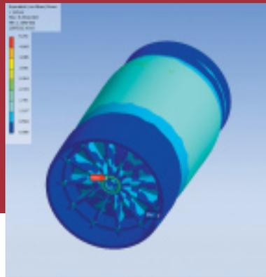
**Right:** After the iterative process of testing various combinations using ANSYS DesignSpace software, the final design included 12 radial ribs with a thickness of 0.125 inch.
