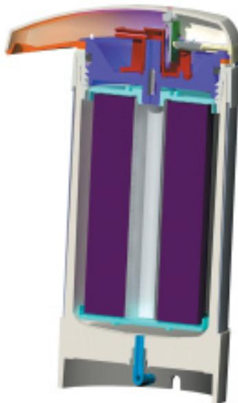
Three-dimensional models of the water filter were designed in SolidWorks and then imported into ANSYS DesignSpace software for analysis of various ribbing configurations and wall thicknesses.
