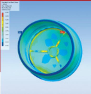
**Left:** In spite of the device's 0.27 inch-thick bottom wall and three internal ribs, stress-levels in the original design were excessive. This showed up as red areas on the ribs, as displayed in this color-coded stress plot.
