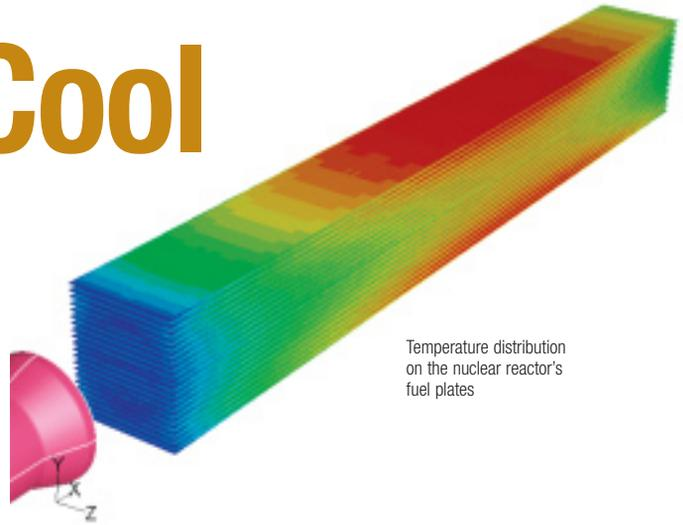
Temperature distribution on the nuclear reactor's fuel plates
