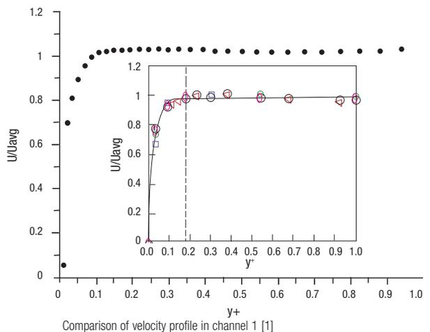
Comparison of velocity profile in channel 1 [1]
