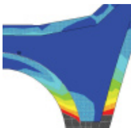
Contour plot of stresses induced by the interference fit between the prosthesis and the bone; the areas colored in grey illustrate the region of the bone that could be expected to yield during the assembly process.
