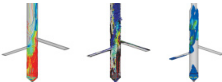
Visualizations of the flow in the mixing zone of the PSDF gasifier for a case with air-blown and steam-enhanced lignite fuel. Included are flow pathlines colored by CO fraction (left); velocity vectors on isosurfaces of solid fraction of 0.2 and 0.3, in which the formation of particle clusters can be seen (center); and contours of carbon reaction rate (right).
