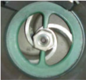
In a Vaughan chopper pump, the main impeller vanes extend all the way to the center hub of the impeller, and the suction plate includes two stationary fingers that protrude to the center of the suction opening. As the main vanes pass by the stationary fingers, a chopping action results, which macerates any solids entering the pump.
