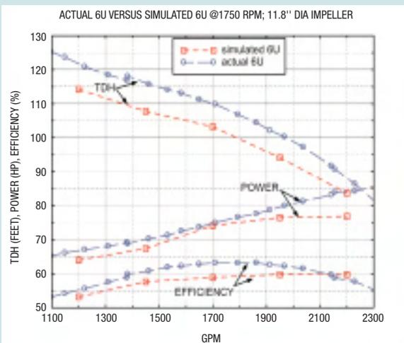
Performance curve for a recently redesigned 6-inch pump. The simulation slightly underpredicts TDH because the geometry for the impeller and casing had to be reverse-engineered, and there were likely some differences between the model and the actual parts.
