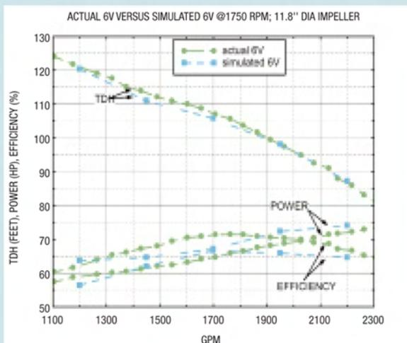
Comparison of the simulated redesigned impeller with the actual redesigned impeller test results show the TDH curves matched very well. Efficiency exceeded expectations, probably because very conservative simulations were run that slightly overpredicted the power required.
