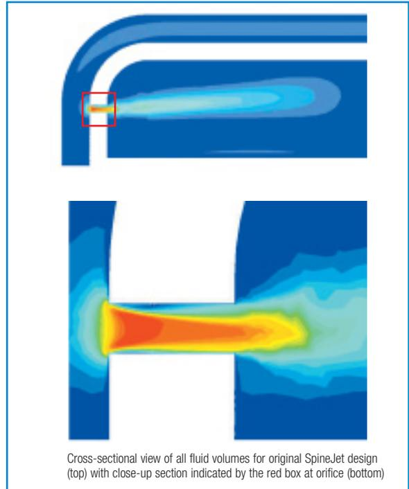
Cross-sectional view of all fluid volumes for original SpineJet design (top) with close-up section indicated by the red box at orifice (bottom)
