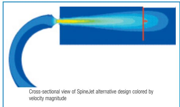
Cross-sectional view of SpineJet alternative design colored by velocity magnitude
