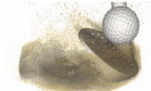
Close up of a golf ball deforming after being struck in a fluid structure interaction simulation, computed using ANSYS AUTODYN software
