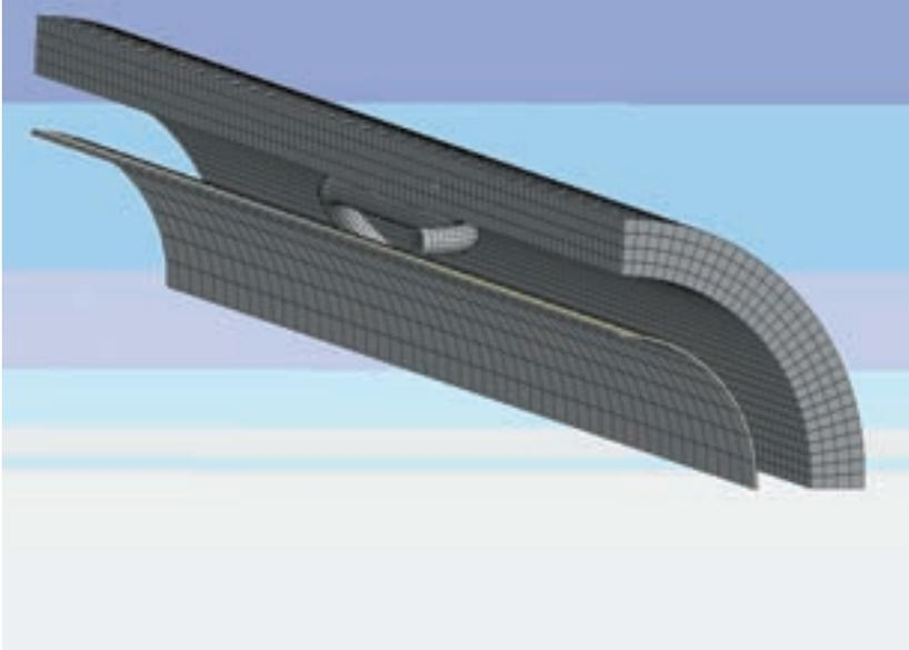
The detailed ANSYS model includes elastin and collagen fibers for the artery, a hyperelastic model for the balloon and an isotropic model for the stent.
