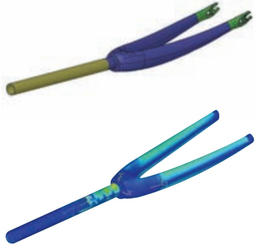
Component geometry from a SolidWorks CAD model (top) was imported into ANSYS Mechanical software (bottom) to determine the stresses in the fork assembly made of aluminum and composite parts. The simulation reduced the number of lengthy hardware prototype iterations and enabled the company to meet critical product launch deadlines.
