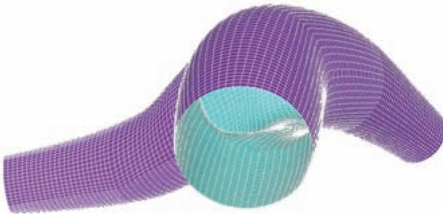
Mesh generated using ANSYS ICEM CFD Hexa; the CFD domain is bounded by the blue cells and the shell mesh, used for the structural calculation, is shown in lavender.
