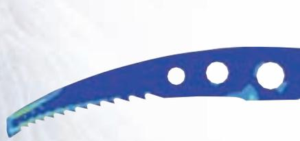
The first principal stress 4.6ms after the initial impact in a transient FEA analysis; the highest tensile stress is apparent at the root of the teeth.
