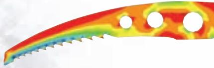
The above two figures show the third principal stress 1.6ms after impact in a transient FEA analysis and depict the most compressive stresses at the root of the axe teeth; the stress shown is above the yield stress of the material, so any tensile stress present at a later time is a residual stress.
