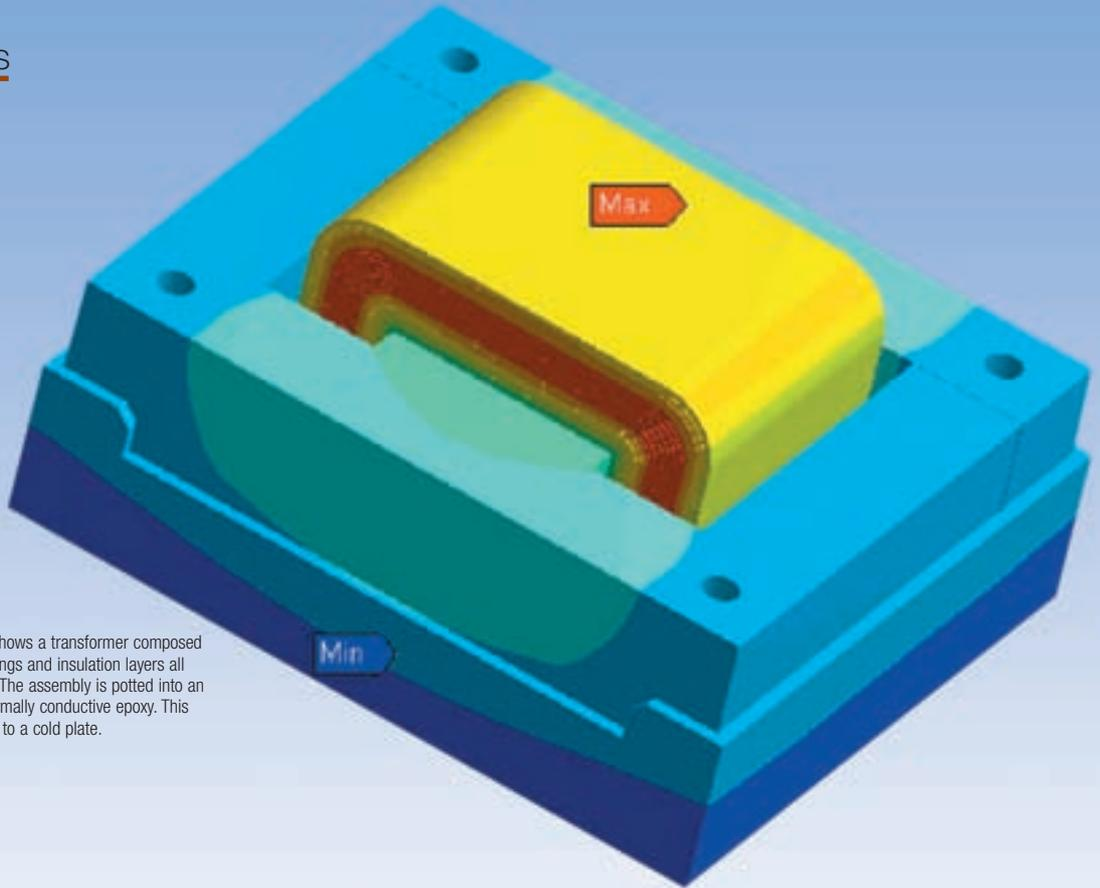
This MatWeb application shows a transformer composed of steel core, copper windings and insulation layers all spiraled into an assembly. The assembly is potted into an aluminum case with a thermally conductive epoxy. This assembly is then mounted to a cold plate.
