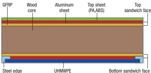
Cross-section schematic of a ski's sandwich structure. Image courtesy Stöckli Swiss Sports AG.
