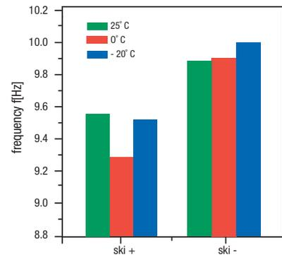
Comparison of the first resonant frequency of *ski+* (left) and *ski-* (right) at different temperatures. These measurements were carried out using accelerometers placed on the ski. The added weight of the accelerometers reduced the resonance frequencies somewhat but had no effect on the relative influence of the topsheet.
