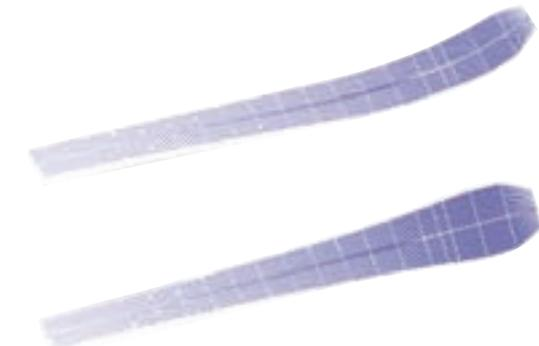
Images generated by FEA for (top) the second flexural mode of the front part of a ski and (bottom) the first torsional mode
