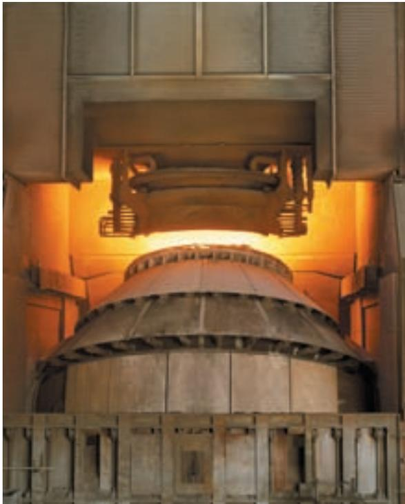
A basic oxygen furnace converter in operation
