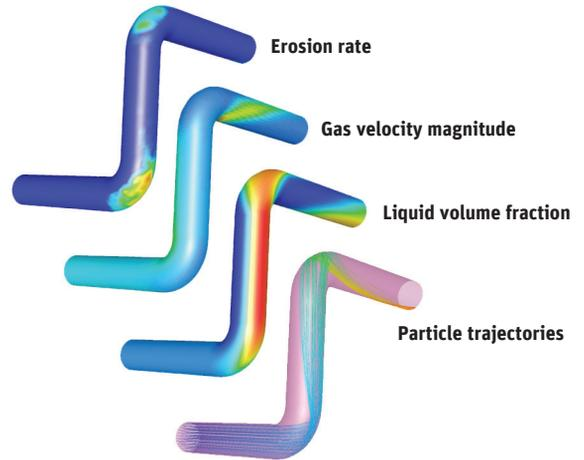
▲ Contours of volume fraction in three-phase analysis to better understand pipeline erosion
