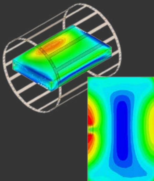
MRI safety simulation for implanted metal stents
