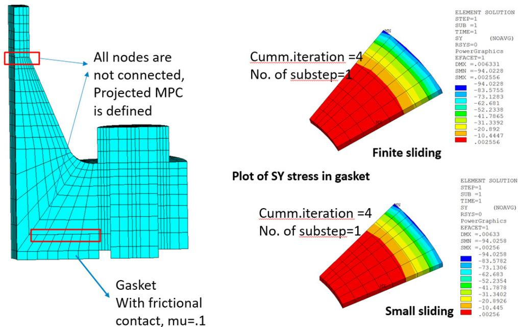
However, the small-sliding logic can cause nonphysical results if the relative sliding motion does not remain small. You must therefore ensure that the small-sliding assumption is valid throughout the analysis.
