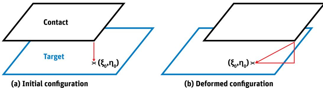
Gap and slip are measured from the contact detection point to its original nature coordinator of intersection on target.
