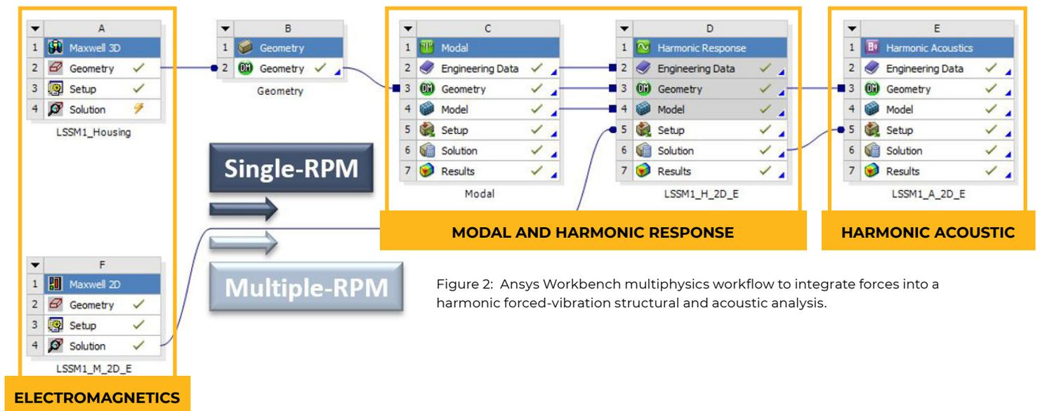
Figure 2: Ansys Workbench multiphysics workflow to integrate forces into a harmonic forced-vibration structural and acoustic analysis.
