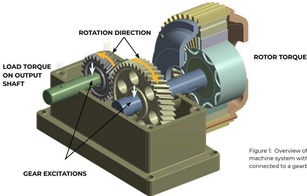
Figure 1: Overview of an electric machine system with the motor shaft connected to a gearbox.
