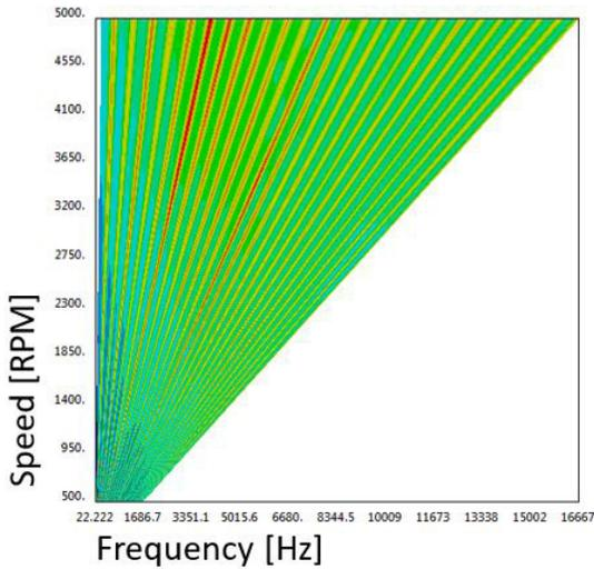
Figure 3: Equivalent Radiated Power (ERP) waterfall diagram showing ERP versus speed and frequency.
