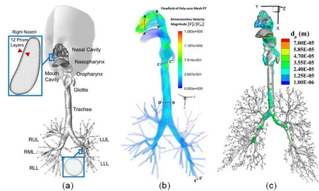
Figure 2. Examples of numerical setup and outputs: (a) subject-specific airway and CFD mesh, (b) airflow field visualization; and (c) droplet deposition with diameter changes
