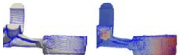
Figure 4 – (Left) Distortion Compensated simulation results in blue superimposed upon the STL file in gray. (Right) Simulated distortion without distortion compensation in blue and red superimposed on the scanned after cutoff results compared to scan data. ANSYS Additive Print accurately predicted distortion for both cases and provided an STL to correct distortion for this geometry
