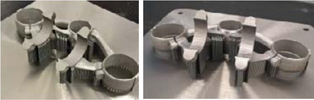
Figure 2 - Bike stem builds. (Left) Non-Compensated Part. (Right) Compensated Part.
