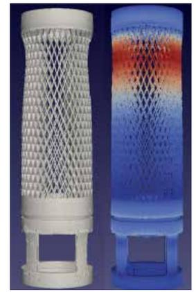
Figure 5: (Left) Distortion compensated STL file at 1.0 magnitude. (Right) Predicted final shape after build of distortion compensated geometry.
