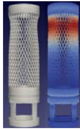
Figure 5: (Left) Distortion compensated STL file at 1.0 magnitude. (Right) Predicted final shape after build of distortion compensated geometry.
