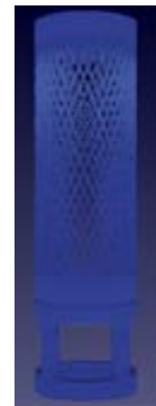
Figure 6: Simulation results of two iterations of distortion compensation at a factor of 0.5.
