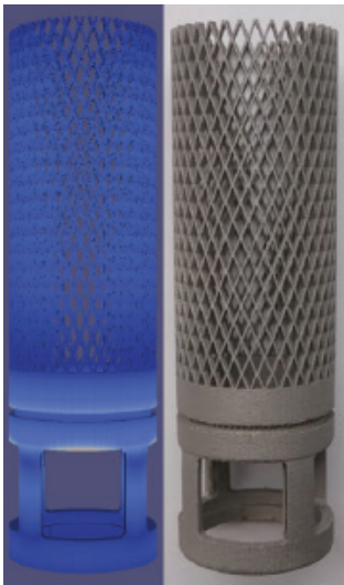
Figure 2. Simulation and physical build images showing no bulge before top ring is added
