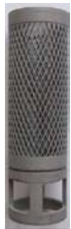
Figure 7: Physical build of 1.0 magnitude distortion compensated file showing no external bulge and nearly vertical walls.
