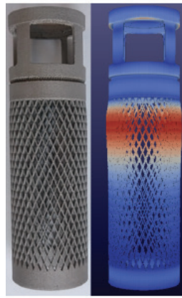
Figure 4. Simulation accurately predicted that the bulge in an inverted filter will occur in a different portion of the mesh region, just below ring.
