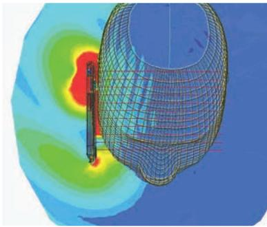
▲ 2-D radiation pattern of conventional omnidirectional cell phone antenna calculated by ANSYS HFSS
