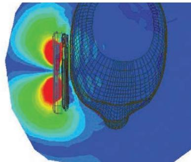
▲ 2-D radiation pattern of Vortis antenna calculated by HFSS . Reduced amount of red at the head indicates a better-distributed signal.
