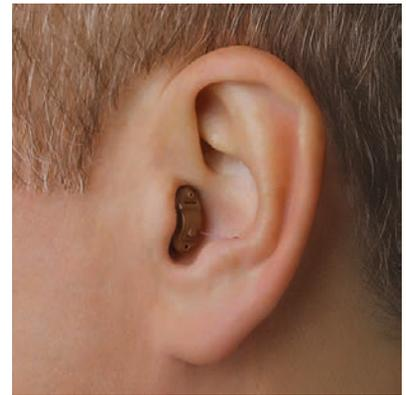
▲ For hearing aids worn in the ear, all the components must fit within a package that accommodates the smallest ear size.
