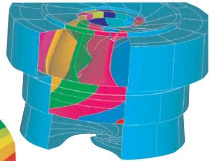
ANSYS model of a hydraulic turbine (top) and FLUID30-based pressure field (bottom)
