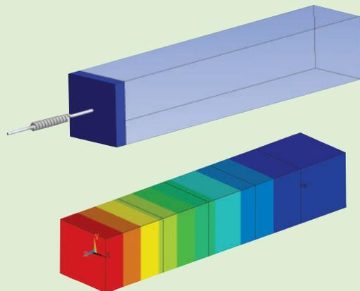
Gases add stiffness to the containing structure, as in the piston shown here supported by a spring and an attached air enclosure (top) with an uncoupled dry mode at 40 Hz and a coupled wet mode at 80 Hz. Pressure mode of the cavity (bottom) was found using ANSYS FLUID30 elements to analyze the system.
