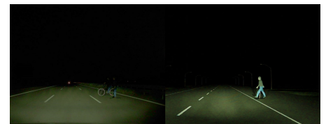
Real image at night taken with Continental's front camera (left) and same camera model in Ansys AVxcelerate Sensors taken in virtual environment (right).
