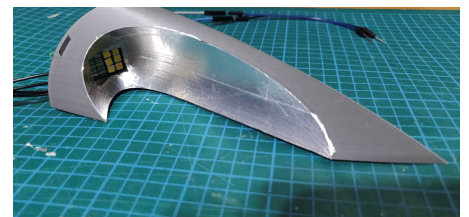
Figure 4: 3D printed prototype of the right Daytime Running Light reflector
