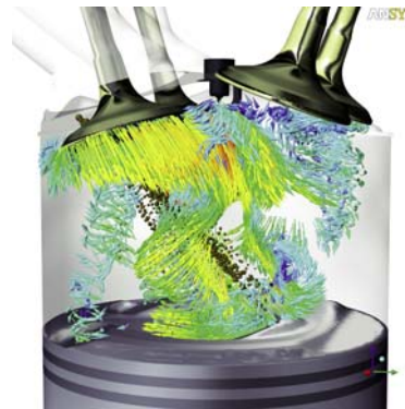
Figure 11: Vortex structures in a GDI engine. Courtesy BMW Group
