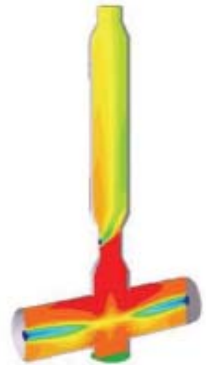
Figure 4: Contours of temperature computed inside the gasifier, with red representing the highest value and blue the lowest
