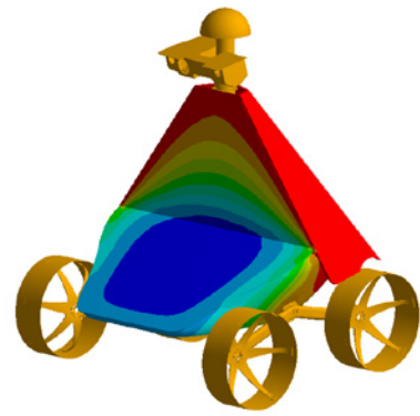
Steady-state thermal study shows temperature distribution on the radiator and surrounding panels used to dissipate excess heat generated by the robot.
