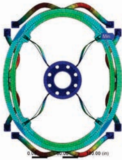
Telescope and camera assembly at mode 6 natural frequency of 14.006 Hz
