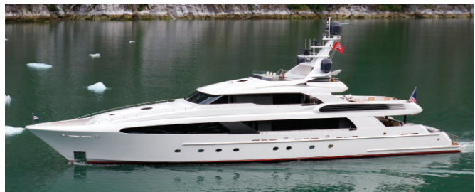
Mr. Terrible cruising Alaska. This 154-foot semi-displacement design is built for high-performance, reaching maximum speeds of 24-knots. Photo by Neil Rabinowitz.
