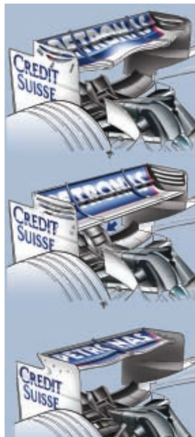
Aerodynamicists tune the configuration of the rear diffuser to provide different downward force strength depending on characteristics of individual tracks. Top to bottom shows designs used in the 2007 season for races at Montreal, Canada; Barcelona, Spain; and Monza, Italy.
