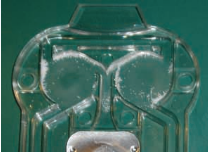
Sweeper particle retention within classifier chambers (approximately 175 micron particles)
