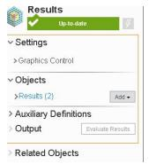
d. Now we can see the results by click on the word <u>Results</u> in this panel. Doing this will bring up another menu with two items, <u>Equivalent Stress</u> and <u>Displacement Magnitude</u>. <u>Clicking the arrows located in the top-left</u> will allow you to navigate between the two results.
