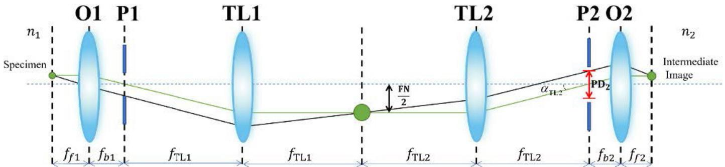
Figure 1. Principal ray and ray just passing the edge of the limiting aperture, traced through the remote refocusing system. Here, the limiting aperture at P1, and the image of the limiting aperture is indicated in the P2 plane in red. O: objective; TL: tube lens; ff and fb : front and back focal length; FN: field number; P: pupil plane; n: refractive index; and PD: pupil diameter.
