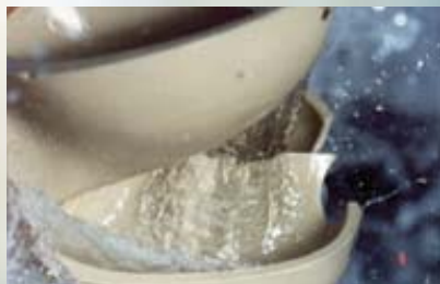
Jet visualisation of a Pelton turbine in hydraulic laboratory.
