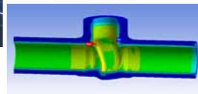
Power plants with aging boilers and piping systems face expensive shutdowns due to service-related damage. Structural Integrity Associates used ANSYS software to analyze thermal fatigue and creep in power plant valves, avoiding unnecessary valve replacements while keeping the plant operating safely.
