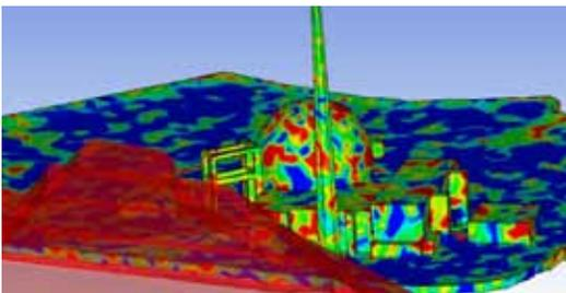
Eletronuclear S.A. simulated potential damage from a hypothetical external explosion at a nuclear plant. Using ANSYS explicit tools, the team gained insight on how to mitigate damage; it also obtained required clearances for plant licensing and construction without performing expensive experiments.
