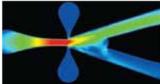
The University of Sheffield is exploring ways to reduce CO<sub>2</sub> emissions through algae-derived biofuels. Researchers applied our software to create an oscillator that produces microbubbles. The system provides greater mass transfer rates, which might translate into higher yields and lower costs in biofuel production.
