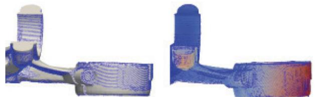
Figure 4. (Left) Distortion-compensated simulation results in blue superimposed upon the STL file in gray. (Right) Simulated distortion without distortion compensation in blue and red superimposed on the scanned after cutoff results compared to scan data. exaSIM accurately predicted distortion for both cases and provided an STL to correct distortion for this geometry.
