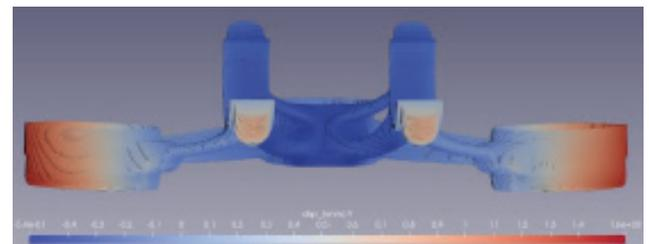
Figure 3. After cutoff displacement simulation results
