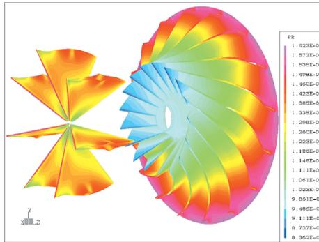
CFX calculates force and torque from pressure and viscous shear stress on the surface of inlet guide vanes and impeller of a Trane centrifugal compressor stage.
