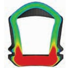
Velocity profile across a die land inlet section. Using the inverse die design capability of ANSYS Polyflow software, the die land can be automatically created to generate the correct extrudate after all deformations.
