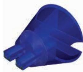
Fluid model extracted from solid CAD model
